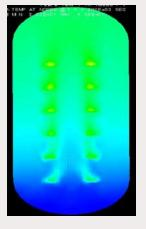
Figure 2,3,4: TWS hot water cylinders are specially designed for heat pumps. In the photograph, the hot water is represented by the green colouring and cool water by the blue. The technology layers the hot water in the hot water tank so that the heat can be used in the best way.
